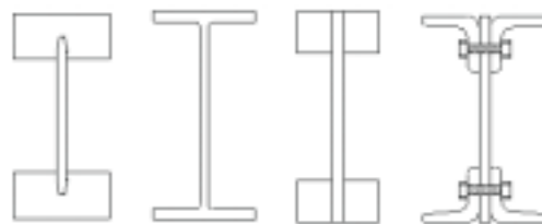
Figure 1 Timber and steel I-joists left: factory produced, right: craft-based
